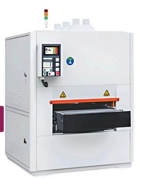
It offers two important functions in the wood processing industry. The first is the calibration process, which makes the material thickness uniform across the entire surface. The second is the sanding function, which prepares the material surface for subsequent processes.
