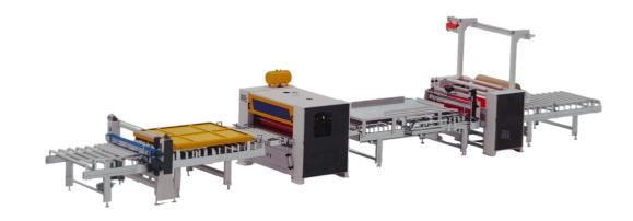
This is a production line that enables high-durability lamination of film or sheet materials onto panels using PUR (reactive polyurethane) adhesive technology.
