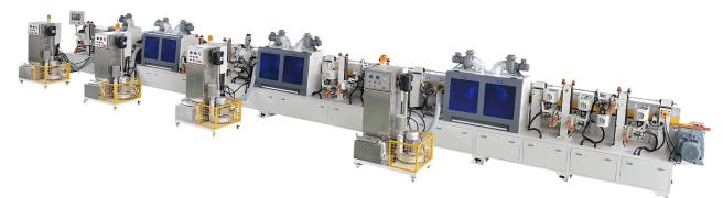
The Edge Painting Machine allows for painting of flat and various shaped furniture, cabinet doors, drawer fronts, MDF, and similar edge materials with UV-based chemicals, using a servo vacuum unit.
