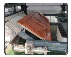
The Cartesian Spray Robot is specifically designed to spray the various panel-type workpieces, like wooden panels, flat & raised door, carved cabinet door, curved panels, stair and other furniture components.
